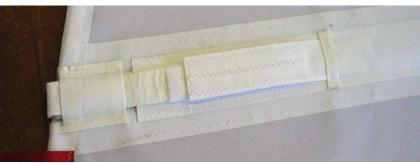
5. Finally press the Top Flap onto the top of the Leech Flap.
