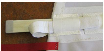
3. Insert the batten through the middle of the loop created by the folded over Leech Flap. Then push the batten all the way into the pocket.
